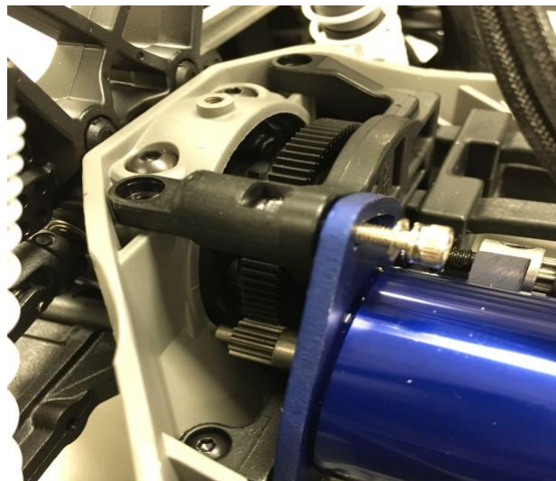
Figure 3.2.1.2: Assembly of the vehicles' stock motor
