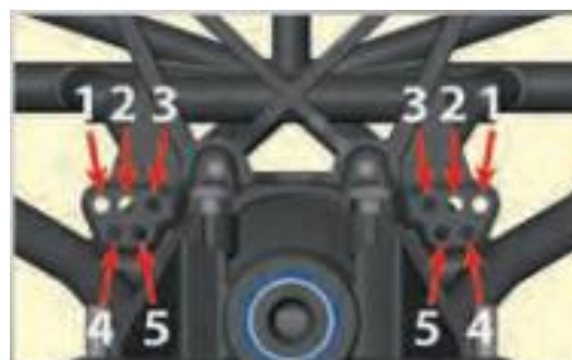
Figure 6.1.3.2: Rear suspension, roll center adjustment point. Source: [125]
