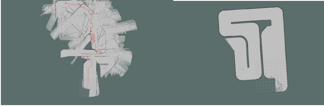
Figure 3.7.2.1: Hector SLAM (left) and Gmapping (right)
